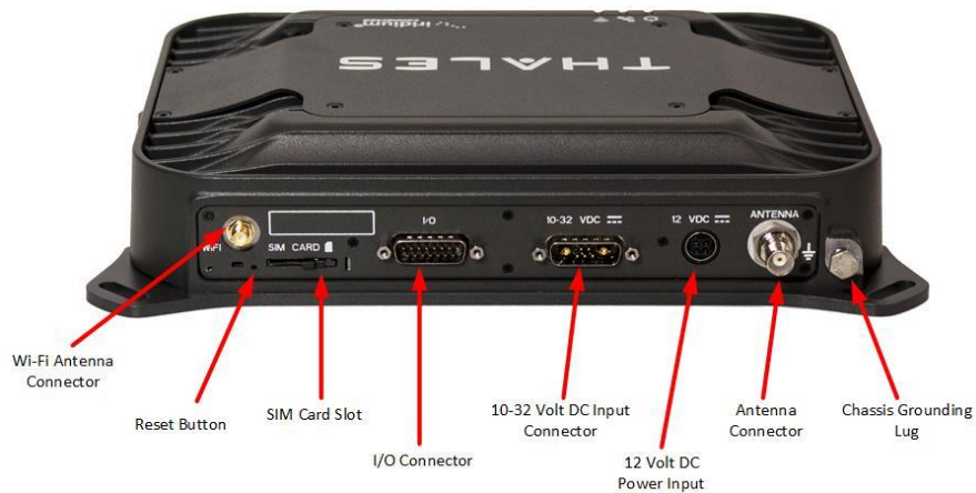
Figure 2-7 Terminal Unit (TU) Back Panel Detail
